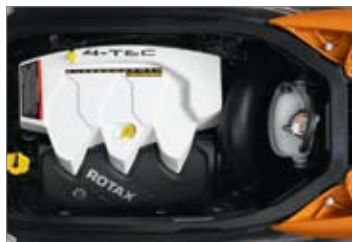
255 hp Rotax 4-TEC engine
